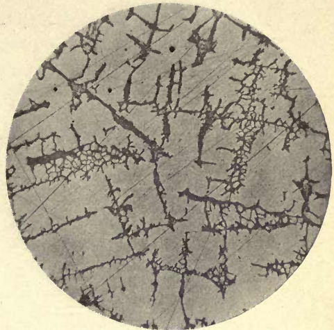
Fig. 37a. \times 40 Alloy 78. Cu 65.0 Slowly cooled in Sn 25.0 furnace. Zn 10.0 \gamma + eutectoid.
